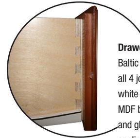
**Drawer boxes** consist of 1/2" 9-ply Baltic birch plywood dove-tailed on all 4 joints. The drawer bottom is white thermo-fused melamine on 1/4" MDF board, captured on all four sides and glued in place. Drawer fronts are applied separately.
