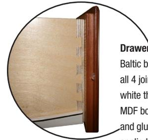
**Drawer boxes** consist of 1/2" 9-ply Baltic birch plywood dove-tailed on all 4 joints. The drawer bottom is white thermo-fused melamine on 1/4" MDF board, captured on all four sides and glued in place. Drawer fronts are applied separately.
