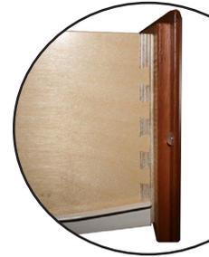
**Drawer boxes** consist of 1/2" 9-ply Baltic birch plywood dove-tailed on all 4 joints. The drawer bottom is white thermo-fused melamine on 1/4" MDF board, captured on all four sides and glued in place. Drawer fronts are applied separately.
