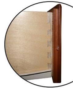
**Drawer boxes** consist of 1/2" 9-ply Baltic birch plywood dove-tailed on all 4 joints or 1/2" thick melamine drawer sides, hardwood doweled in place. The drawer bottom is white thermo-fused melamine on 1/4" MDF board, captured on all four sides and glued in place. Drawer fronts are applied separately.
